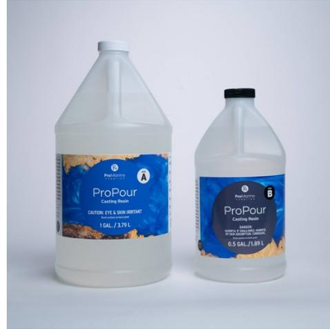
Casting resin’s 2:1 mixing ratio by volume (resin to hardener) is formulated for thicker layers (also known as “deep pours”) of up to 1.5” without the worry of the material overheating. The slightly thinner viscosity, as compared to other resin types, provide longer working times and slower/cooler cures.
