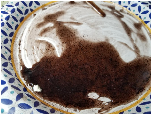
Epoxy resin mixed with wood shavings for tint
